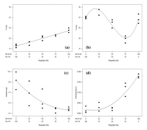
Figure 1. Flow Ability and Compressibility Value (a. T.I Dry Mixture; b. T.I CPE; c. Hardness Dry Mixture; d. 1/Hardness CPE)
