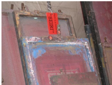
Figure 1- Tags are used to identify the places where a particular 5S activity is required. Change the tag color for each activitylike Red for SEIRI, BLUE for SEITON and Green For SEISO.
