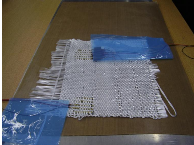
Figure 10b layered piezofilm woven into composite preform prior resin infusion.
