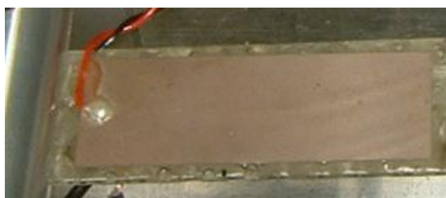
Figure 2 PZT coupon laminated unto braided composite
