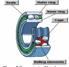
Figure 2 Components of bearing
