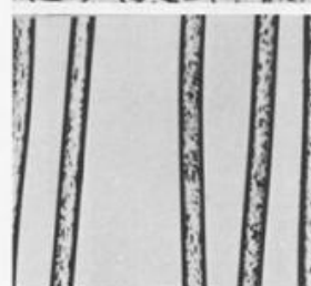
Fig. 21 Polyester, Regular melt spun, 3.0 denierper filament, semi dull
