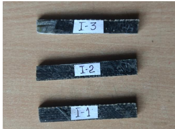
Fig. 2&3 Tensile and impact test samples
