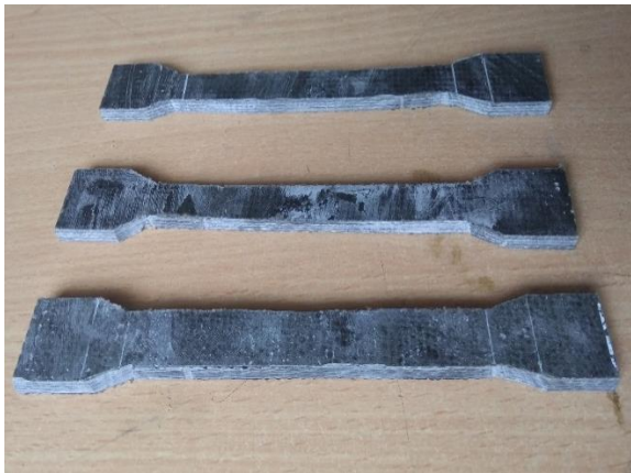
Fig. 2&3 Tensile and impact test samples
