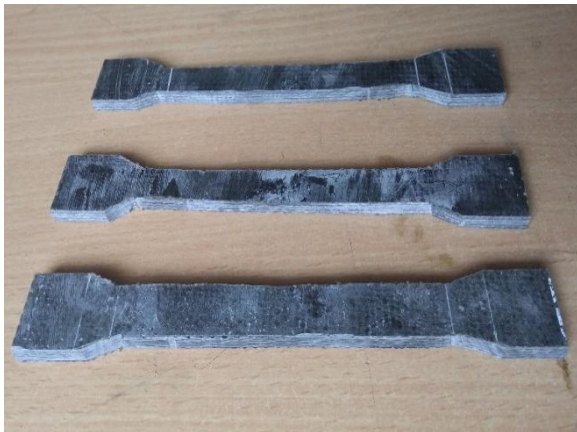
Fig. 2&3 Tensile and impact test samples
