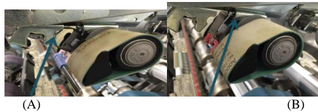
Fig.6. Old spring (A) and new spring (B).
