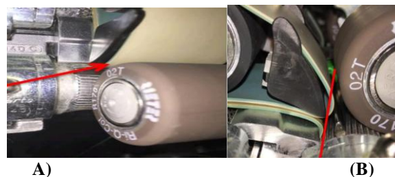
Fig.8. Correct setting of nose bar and cradle.
