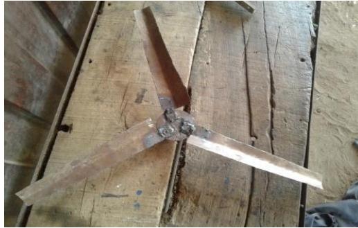
Figure 2: constructed Turbine (3-dimensional blade)
